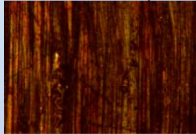
Wear pattern on the test disc - 100 x magnification
